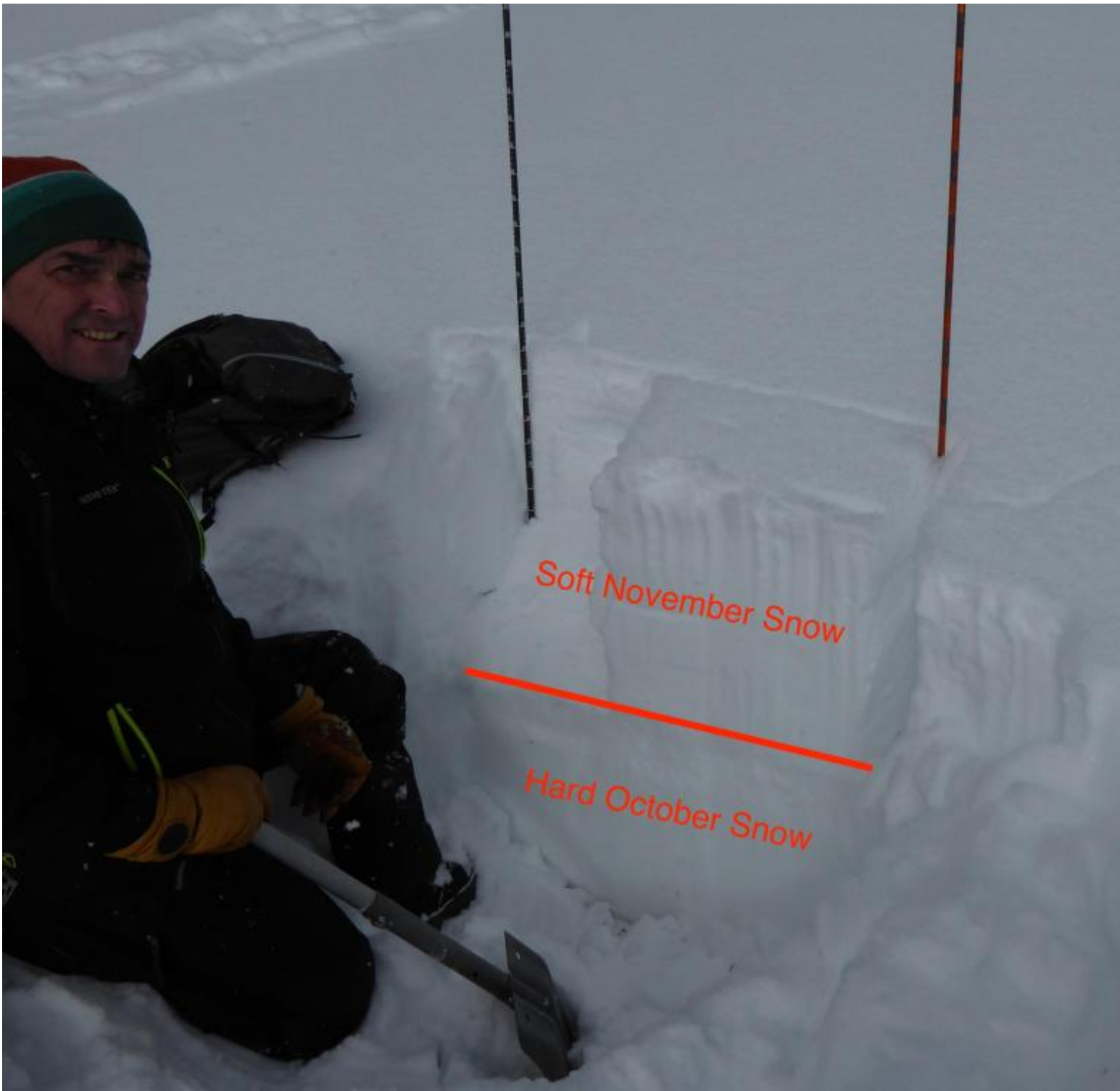
A south facing snow profile near Lulu Pass in Cooke City. The bottom half of the snowpack is hard October snow. The top half of the snowpack is soft November snow. No propagation in an Extended Column Test. Photo: GNFAC
