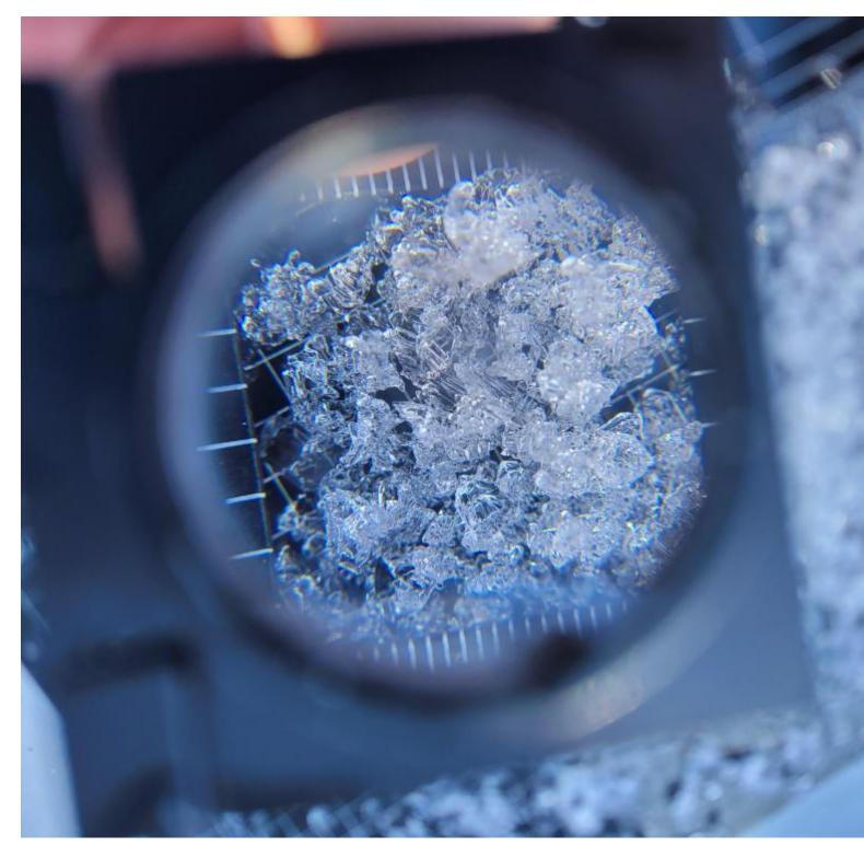
From obs (4/18/21): "...class split and dug three pits, one on NE, one on N, and one on NW at 7623'. HS averaged around 70 - 100 cms... The NE and NW facing pits showed rounding depth hoar and no sudden CT results. None of the ECTs fractured or propagated. The N facing slope still had preserved advanced depth hoar 3 mm in size (see image)..." Photo: J. Quinn
