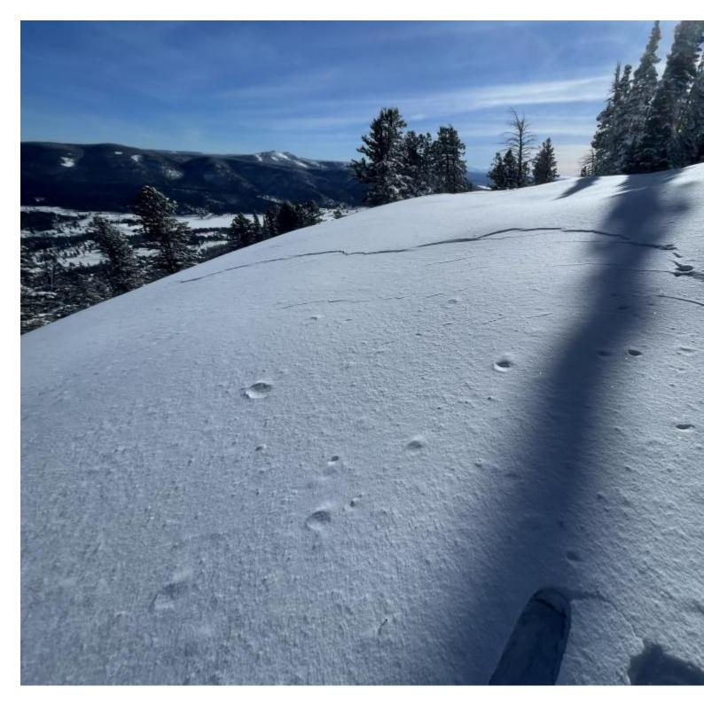
From obs: "We observed widespread shooting cracks on all ridges and all NE facing slopes. Cracks would propagate up to 200' in front." O. Robinson
