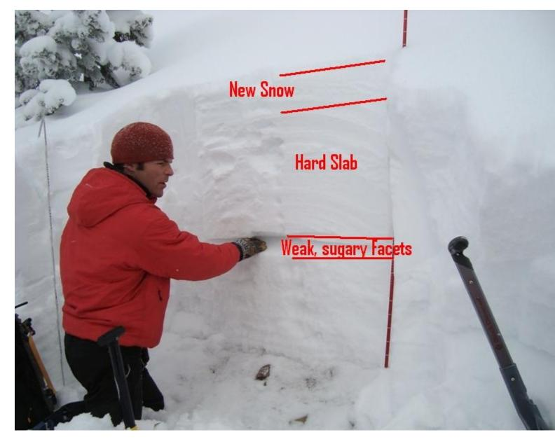
Mark Staples points out the weak layer that the avalanche ran on. Large faceted grains, formed by the cold temperatures in early December, was the layer that failed. These sugary grains were overburdened with a thick hard slab 2 feet thick.
