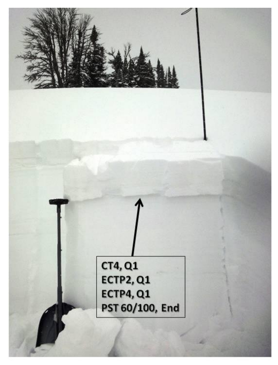
This snowpit was dug on an east facing, 35 degree slope at 9,000 feet. The break occured 20 cm down on lower density stellars crystals that fell two days ago. I do not anticipate this weakness to last more than a few days. Photo: GNFAC
