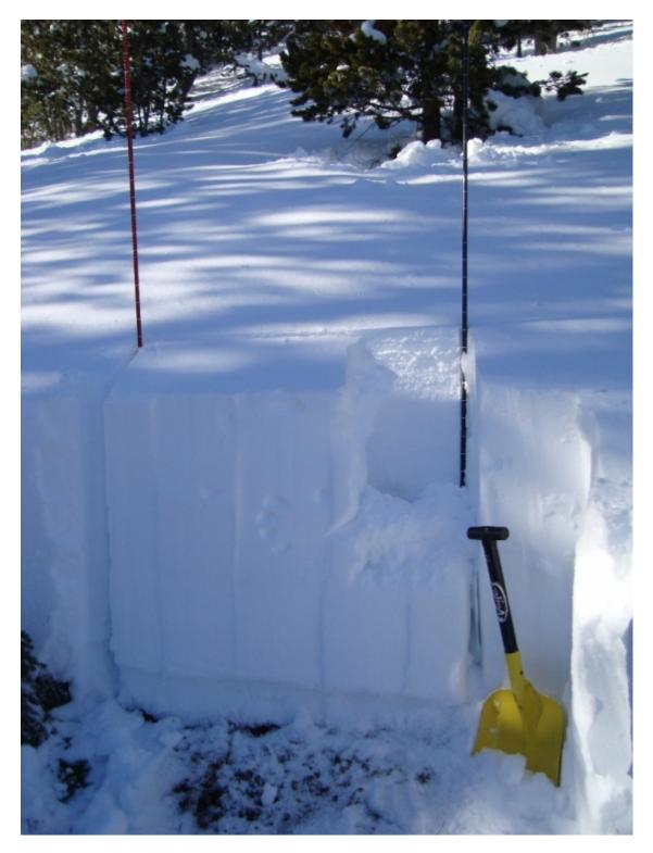
This three foot deep snowpack was breaking near the ground on facets. ECTP22,Q1 was our test score. The pit was at 9,330 feet on a southeast facnig slope. We were not excited to find the weak snow propagating fractures and we stuck to terrain that was not exposed to avalanches. Photo: GNFAC
