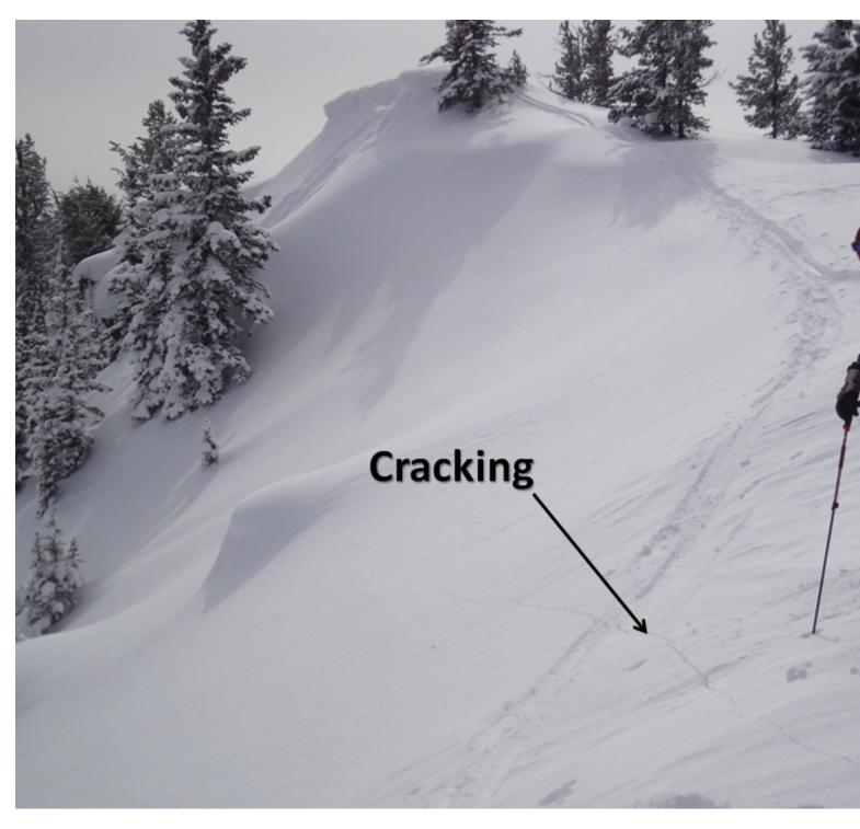
At the ridgetopp near Hebgen Lake, about a few hundred feet above our snowpit where we got ECTP20, Eric got a large collapse and cracks. In this zone the near surface facets about 1.5 feet under the surface are propagating fractures. Photo: GNFAC
