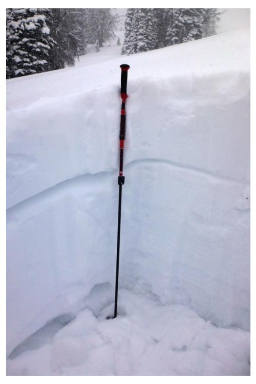
The 40cm of new snow is now capping the 5cm thick layer of small grained facets. The stripe in the pit wall is where the facets are located. CT12/ECTP14 on this layer. More snow will likely create natural avalanches. This pit was dug above Hebgen Lake, but the snow structure is similar to most of our area. Photo: GNFAC
